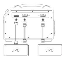
1. Before connecting, please check whether the terminals and wiring harness of the battery pack are damaged or disconnected; 2. When using the adapter cable, be sure to connect according to the positive and negative signs.
